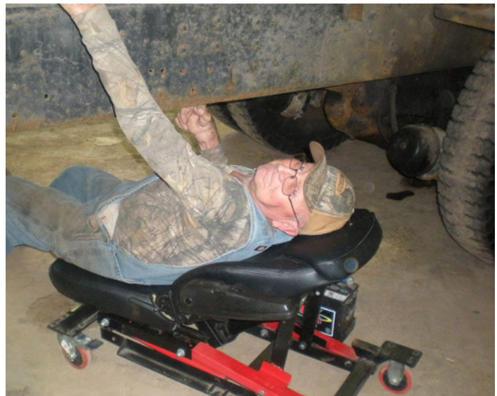
Figure 43. This 12V powered work positioning seat reclines and powers up and down.
