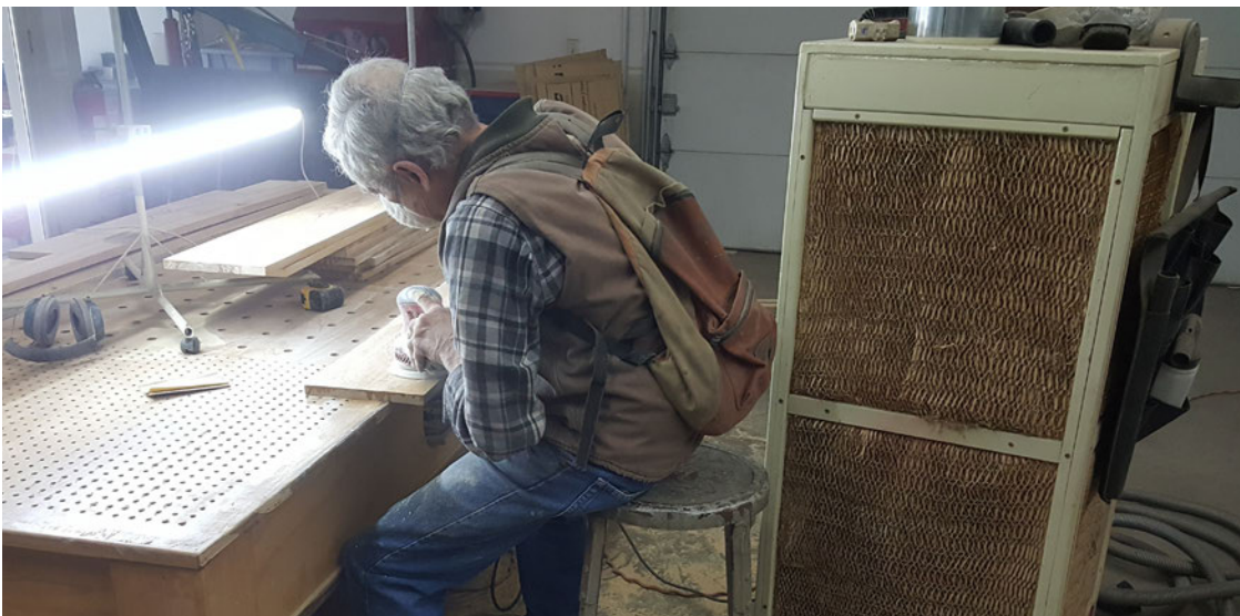
Figure 18. Air cleaner systems draw dusty air through filters and blow the clean air back into the room but require regular maintenance. This table has a vacuum that draws dust down through the holes and into a filter.
