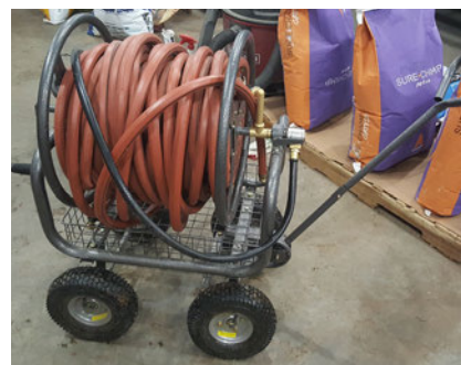
Figure 11. Use a hose reel on wheels to easily store the hose and move it to a warm storage location.
