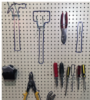
Figure 37. Outlines of tools on a pegboard help workers know where to return tools for regular storage.
