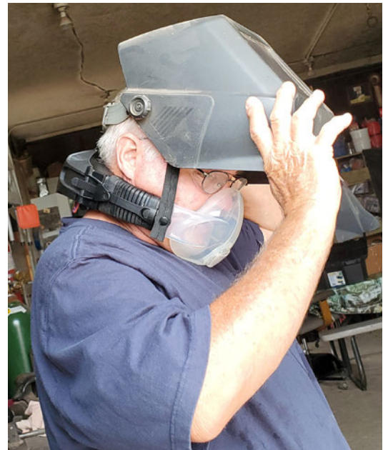
Figure 17. When adequate ventilation cannot be achieved for the workspace, powered air purifier respirators like the Cleanspace respirator will filter fumes and dust from the air for an individual worker. CAUTION: PAPR systems will not protect from oxygen deficient environments or prevent carbon monoxide poisoning!
