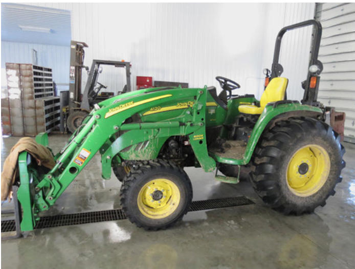
Figure 9. Properly sloped floors and adequate floor drains play a crucial role in reducing slip hazards. Use metal floor drain grates rated to support heavy machinery.
