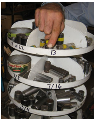
Figure 36. Storing tools in color coded visible places makes it easy to put them away.
