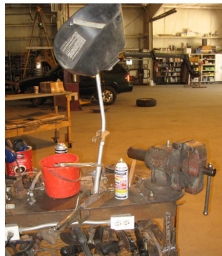
Figure 47. This welder’s workstation has a face shield holder, tools underneath, and electrical outlets.
