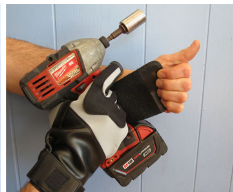
Figure 34. Velcro grip gloves hold the hand in a tight fist without exerting muscle strain. This can be helpful when holding shop tools for long times. This 18V impact driver is a flexible tool for removing fasteners quickly.
