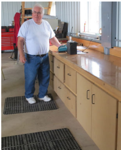
Figure 41. Floor cushions in the workspace relieve hip and back pain. Note electrical outlets along the work bench.
