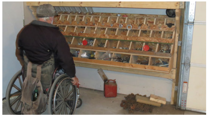
Figure 48. Open bins with labels allow a quick visual scan to find hardware and supplies and identify needed restocking.
