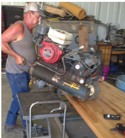
Figure 46. This air compressor was raised from floor to table height with this foot-pumped hydraulic lift cart without straining the farmer’s back.
