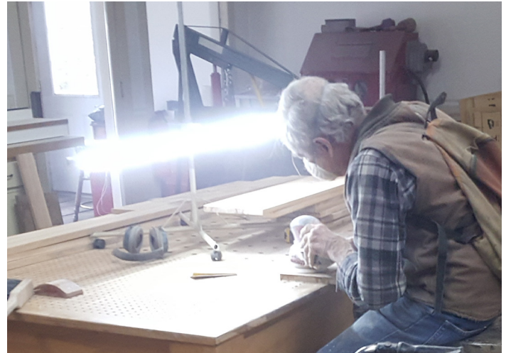
Figure 23. This farmer created an adjustable-height LED light stand to improve visibility in his farm shop.
