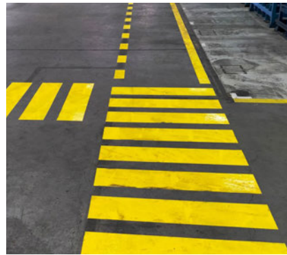
Figure 10. Floor markings keep travel areas clear and can assist workers with low vision when backing equipment into storage or service areas.
