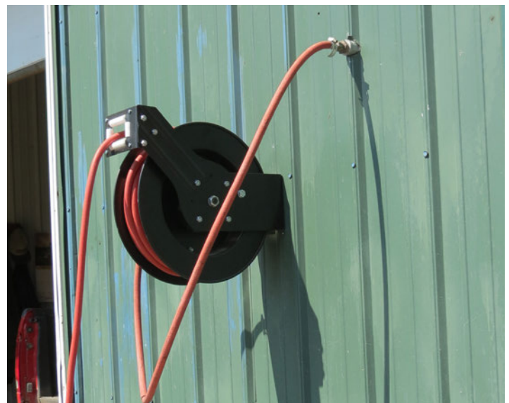
Figure 27. Auto rewind air-line storage reels make it easier for workers with arm impairments to store hoses. They are often mounted on the ceiling or side walls to reduce tripping hazards.
