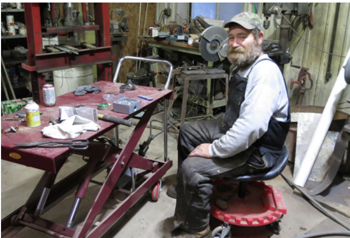
Figure 44. This farmer uses his hydraulic lift cart as an adjustable height worktable. In conjunction with his adjustable height shop stool, he can always work on a project from an ergonomic position.
