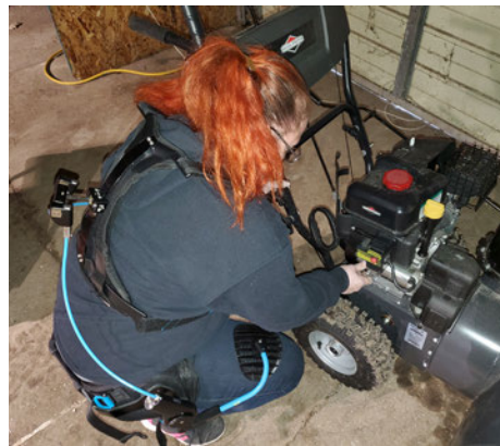
Figure 42. Wearable exoskeletons can support a person's back or shoulders while doing shop work.
