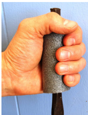
Figure 33. Hand tools with larger cushioned grips and wearing anti-vibration gloves help workers with carpal tunnel and hand impairments.
