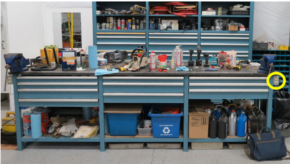
Figure 25. An electrical outlet on the front side of this work bench gives convenient access to power without using extension cords.
