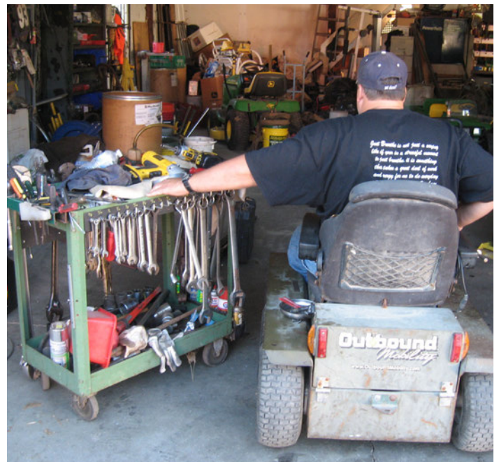
Figure 8. The farm shop will be most accessible when there is plenty of room to push a tool cart around equipment parked inside for repairs.
