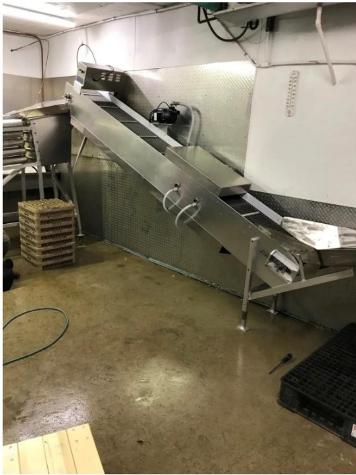
Photo of the washer, conveyor, and counting machine.
