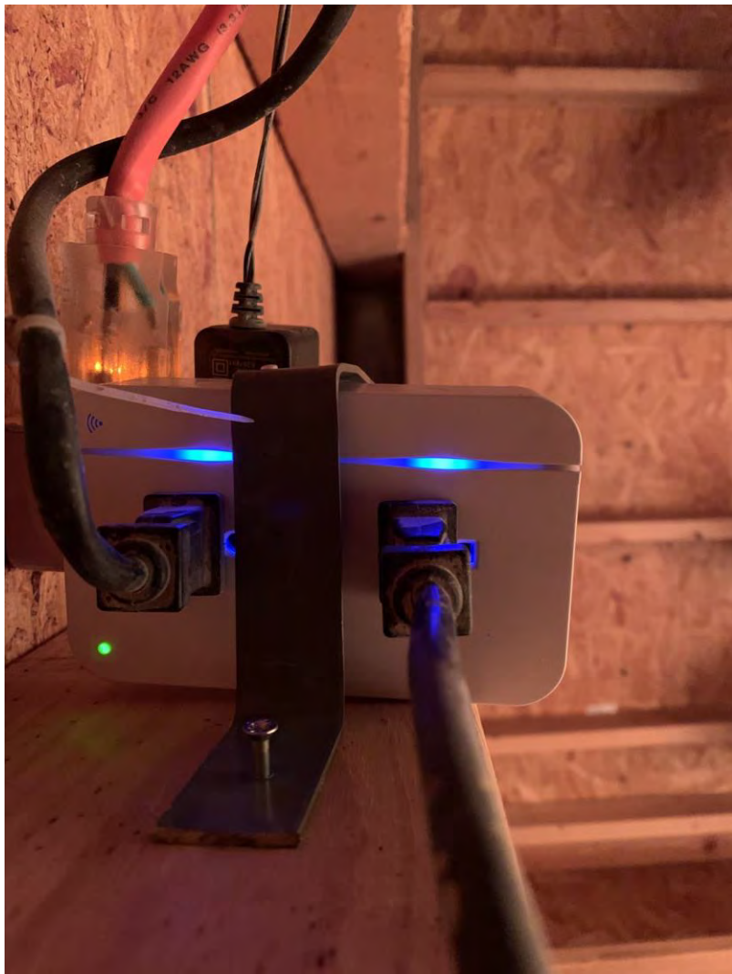
ConnectSense - 2-Smart Outlet Plug powered by extension cord to operate 2 heat lamps in chicken coop.
